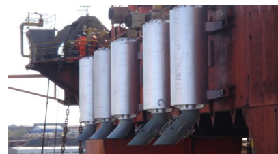
AISI 316 silencers on rig Transocean Searcher
